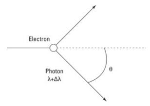
Figure 1-6: Photon scattering off an electron.
