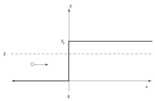
Figure 3-6: A potential step,  $E < V_0$ .
