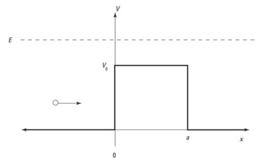
**Figure 3-8:** A potential barrier  $E > V_0$ .
