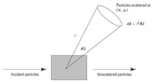
**Figure 12-1:** Scattering from a target.
