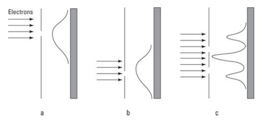
Figure 1-7: An electron beam going through two slits.
