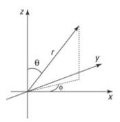
Figure 8-1: The spherical coordinate system.
