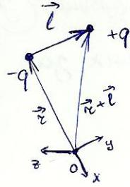
$$W = q\varphi(\vec{r} + \vec{l}) - q\varphi(\vec{r})$$
