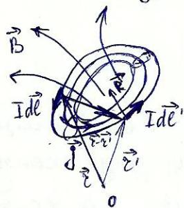
$$\Phi = \int_S \vec{B} d\vec{S} = L I ; \quad \vec{B} = \frac{\mu_0}{4\pi} \oint \frac{I [d\vec{l}', \vec{R}]}{R^3} ;$$
