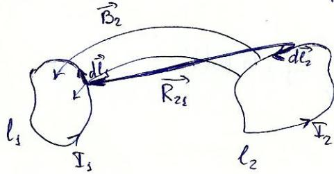
$$\begin{aligned} \Phi_{32} &= \int_{S_{l_2}} \vec{B}_2 d\vec{S}_3 = \oint_{l_2} \vec{A}_2 d\vec{l} = \oint_{l_2} \left( \frac{\mu_0}{4\pi} \oint_{l_1} \frac{I_2 d\vec{l}_2}{R_{2s}} \right) d\vec{l}_2 = \\ &= \underbrace{\left( \frac{\mu_0}{4\pi} \oint_{l_1} \oint_{l_2} \frac{d\vec{l}_2 d\vec{l}_3}{R_{2s}} \right)}_{L_{32}} I_2 = L_{32} I_2 \end{aligned}$$
