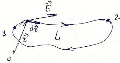
$$\oint_L \vec{E} d\vec{l} = \int_1^2 \vec{E} d\vec{l} + \int_2^3 \vec{E} d\vec{l} = \varphi_1 - \varphi_2 + \varphi_2 - \varphi_1 = 0, \text{ т.е.}$$
