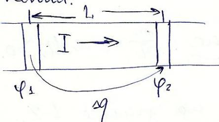
$$\Delta q = I \Delta t, \Delta A = \Delta W = \Delta q (\varphi_3 - \varphi_2) = \Delta q U$$
