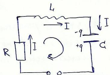
$$L \frac{d^2q}{dt^2} + R \frac{dq}{dt} + \frac{q}{C} = 0 \Rightarrow \ddot{q} + 2\gamma \dot{q} + \omega_0^2 q = 0, \text{ где } \gamma = \frac{R}{2L}; \quad \omega_0^2 = \frac{1}{LC}.$$
