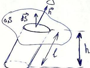
$$\left. \begin{array}{l} \int \vec{E} d\vec{S} = \frac{Q}{\epsilon_0} \\ \int \vec{E} d\vec{S} = E_n \Delta S \end{array} \right\} \Rightarrow E_n \Delta S = \frac{Q \Delta S}{\epsilon_0} \rightarrow \boxed{E_n = \frac{Q}{\epsilon_0}}$$
