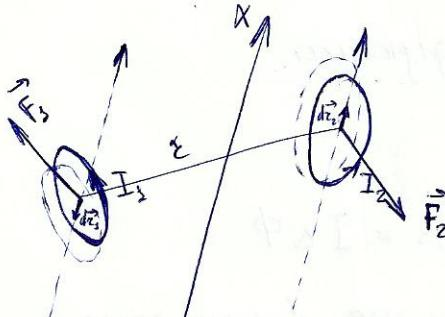
$$F_{2x} = -\frac{\partial U_2}{\partial x_2} = I_2 \frac{\partial \Phi_2}{\partial x_2} = I_2 I_1 \frac{\partial L_{23}}{\partial x_2} ;$$
