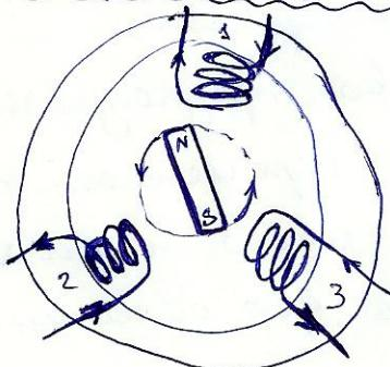
$$E_1 = E_0 \sin \omega t; E_2 = E_0 \sin(\omega t - 120^\circ);$$
