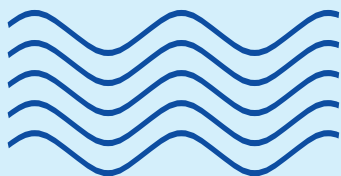
Polymer with few branched chains, e.g., high-density polyethene
