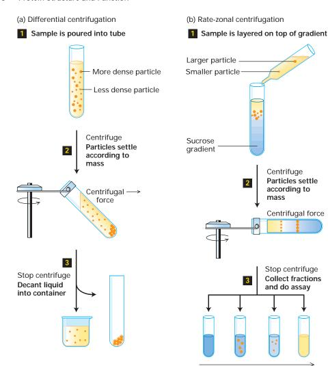
**▲ EXPERIMENTAL FIGURE 3-31** Centrifugation techniques separate particles that differ in mass or density. (a) In differential centrifugation, a cell homogenate or other mixture is spun long enough to sediment the denser particles (e.g., cell organelles, cells), which collect as a pellet at the bottom of the tube (step 2). The less dense particles (e.g., soluble proteins, nucleic acids) remain in the liquid supernatant, which can be
