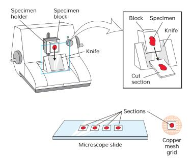
▲ EXPERIMENTAL FIGURE 5-43 Tissues for microscopy are commonly fixed, embedded in a solid medium, and cut into thin sections. A fixed tissue is dehydrated by soaking in a series of alcohol-water solutions, ending with an organic solvent compatible with the embedding medium. To embed the tissue for sectioning, the tissue is placed in liquid paraffin for light microscopy or in liquid plastic for electron microscopy; after the
